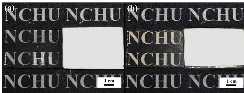
Fig. 11. Photographic images of PET films with the left half coated with (a) artificial brochosome arrays covered with 90 nm hole arrays, and (b) 90 nm hole arrays.
