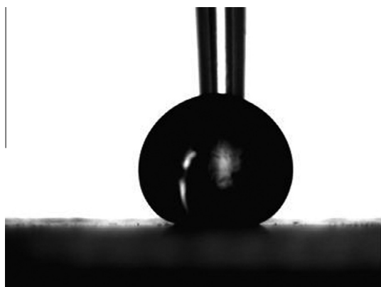
Fig. 5. Water drop profile on a fluorosilane-modified binary colloidal array consisting of 4 \mu\text{m} and 300 nm silica spheres.
